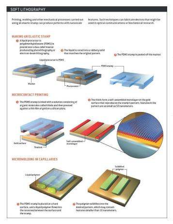
print on planar and non-planar surfaces. The stamp is fabricated from an elastomeric polymer, such as poly(dimethylsiloxane)(PDMS), polyurethanes, polyimide and resins.
