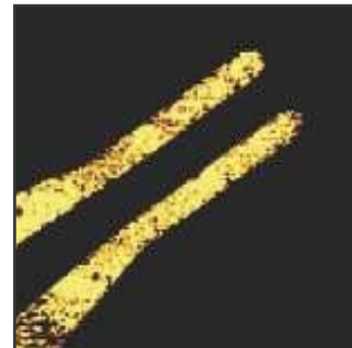
10 x 10 \mu image of silicon sample with gold pattern. At the left is a topography image and at the right is a conductive AFM image. Two of the "fingers" on the test pattern are grounded and show contrast in the conductive AFM image.
