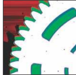
40 x 40 \mu image of a gear fabricated with MEMS.
